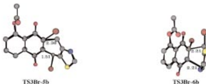
Figure 6. Transition states of the cycloadditions between o -QDM 2 and 2- or 3-bromo-5-acetoxynaphthoquinones 3b or 4b , respectively.
